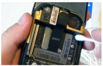
Dampen a cotton swab with water and clean your camera lens and flash using a spinning motion. Once the lens is clean, quickly dry it with the other side of the cotton swab so that water doesn't dry on the lens.
