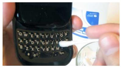
Next move to the rest of the phone plastics. For large areas like the battery cover, it is fine to use rubbing alcohol. Use light pressure when cleaning plastic so you don't remove any rubber coating or clear finish.
